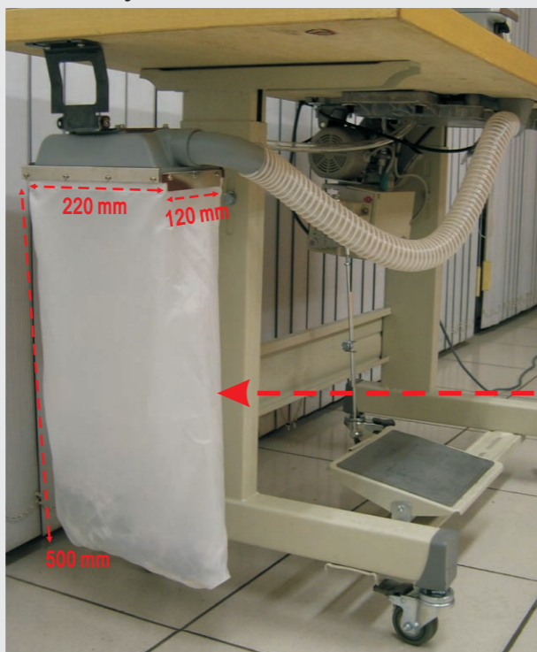
WASTE CAPACITY INCREASE 25%
